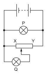
The slider on the potential divider is moved from end X to end Y of the resistor.
